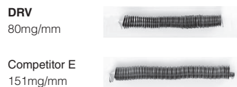
Weight per Unit of Length for Chips Generated by the Inner Edge (Internal evaluation)
